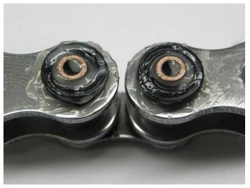
4. Put the plate onto the pins.
