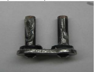
4. Put the pins into the roller links.
