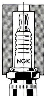
Poor socket design
