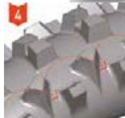
4. Periodic arrangement of 1/2 blocks and shoulder blocks with proper gyration radius (dash line) provides predictable turning and reduced oversteering.
